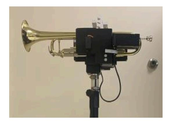
The trumpet assist is designed to hold a standard trumpet on an adjustable stand while providing three low-profile buttons to allow pressing of the trumpet's finger buttons using less force. Two trumpet assist devices have been assembled, one with black and white components for school/concerts and another with blue+white components.
